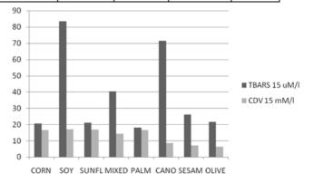
Fig. 3TBARS and CDV values for all the oils studied after 15 min of microwave treatment
